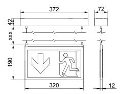
Abmessungen in mm
