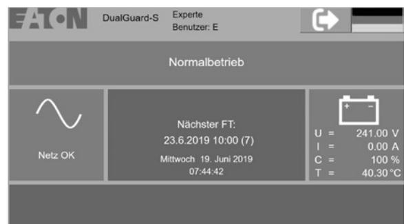
The image shows the main menu of the DualGuard-S system. At the top, it says 'EATON DualGuard-S Experte Benutzer: E'. Below this, there is a 'Normalbetrieb' section. On the left, there is a 'Netz OK' indicator with a sine wave icon. In the center, there is a 'Nächster FT:' section showing '23.6.2019 10:00 (7)' and 'Mittwoch 19. Juni 2019 07:44:42'. On the right, there is a battery icon and a table of system parameters: U = 241.00 V, I = 0.00 A, C = 100 %, and T = 40.30 °C.
